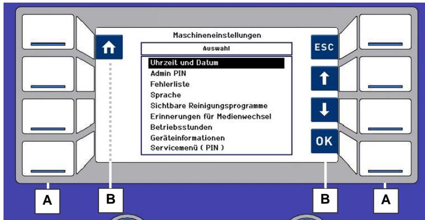
Fig. 3.10.1 Control panel with display and navigation symbols
