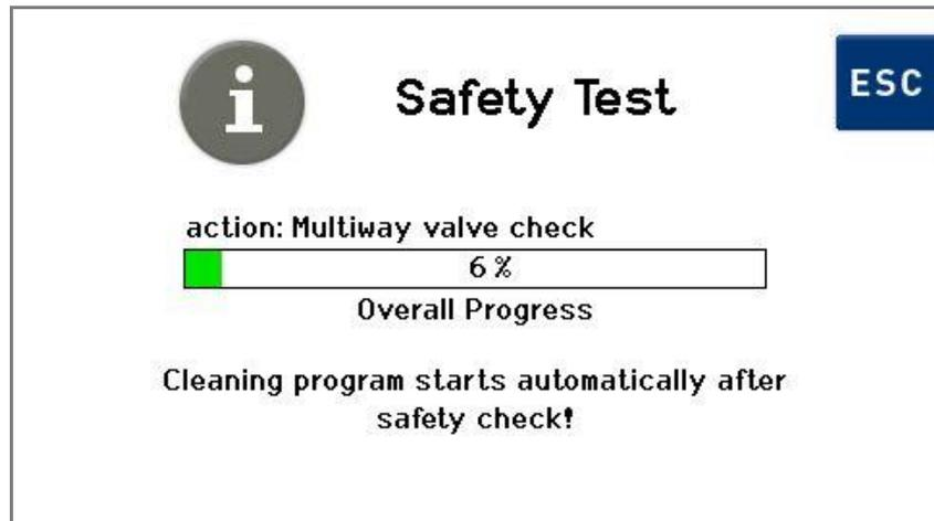
Fig. 6.3.3 Display *Safety test progress*
