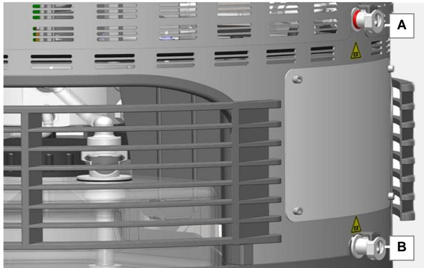
Fig. 14.2.2 Connections for venting
